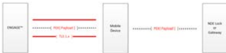
Figure 1: ENGAGE to Device Through MAPP Encryption Diagram
