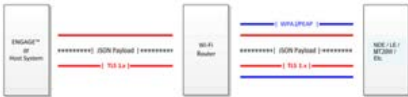
Figure 4: Alliance Partner system to Device Encryption Diagram
